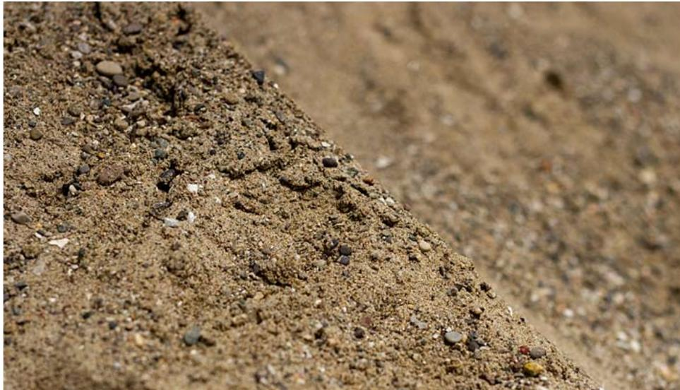
2NS sand, or "sharp sand" as it can be called, is a natural product that has been washed, leaving it free from any foreign debris such as clays and dirt. The sand is 3mm in size and should pass through a #6 sieve, but not a #8 sieve. The sand is not weathered, giving it the "sharper" corners to lock and bind better.
